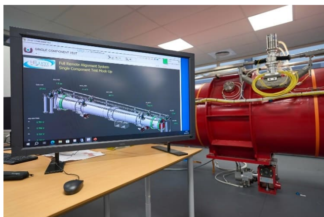
Solutions for the new remote alignment system (FRAS) have been defined and validated using a test model. (Image: CERN)
