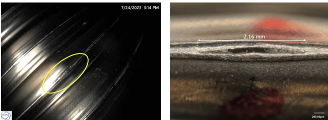
Monday, 24 July, afternoon: SMALL BUT MIGHTY The teams located the M2 bellows that were suspected to be at the root of the problem and, indeed, found that there was a 1.6-mm-long crack on it, which was the source of the helium leak. An action plan was put in place: remove the broken bellows, replace them, do all the necessary tests, close up again and start the cooldown...
